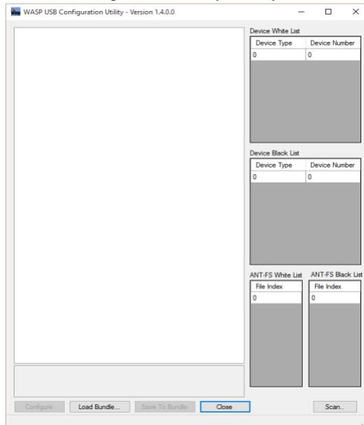
3. Plug the WASP-N into a USB port using a micro-USB cable. The area to the left will fill with the pre-set data read from the WASP-N.
